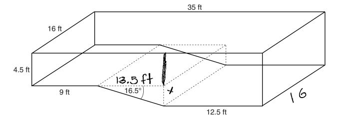
If the sloped floor has an angle of depression of 16.5 degrees, what is the depth of the pool at the deep end, to the *nearest tenth of a foot*?
