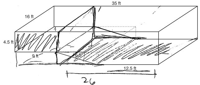
If the sloped floor has an angle of depression of 16.5 degrees, what is the depth of the pool at the deep end, to the *nearest tenth of a foot*?
