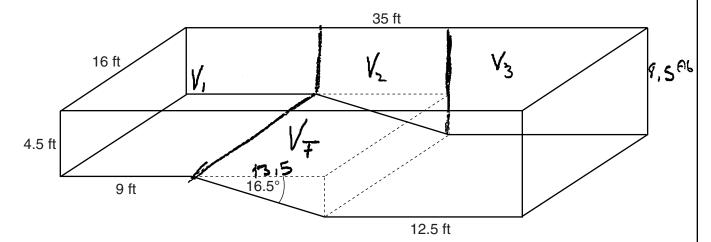
If the sloped floor has an angle of depression of 16.5 degrees, what is the depth of the pool at the deep end, to the *nearest tenth of a foot*?
