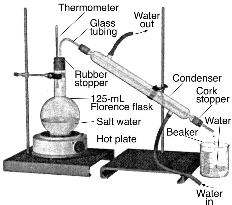
This apparatus is used for which process?
