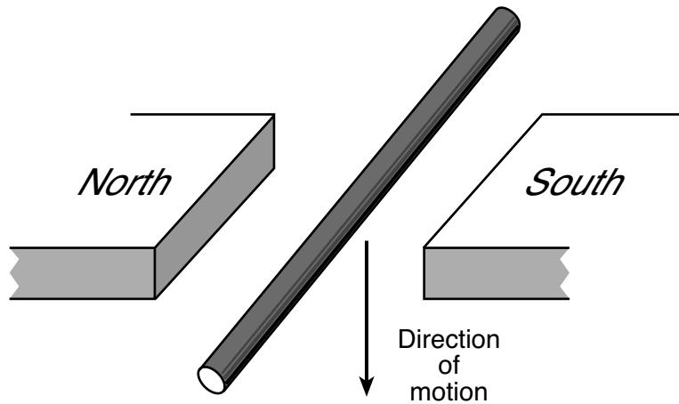
Moving the wire downward between the poles in the direction shown in the diagram will
