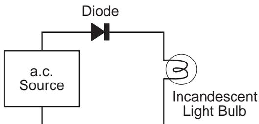
How many times per second does a maximum current exist in the light bulb?
