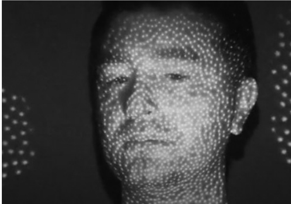
Diagram 3: Infrared Photograph of Projected Dots
